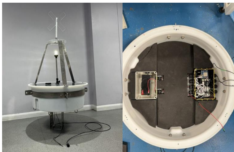
Figure 5.1: Front elevation of the completed prototype, full assembly including tripod, mast, daymark, navigation light, and GPS/4G puck above the inherited hull
